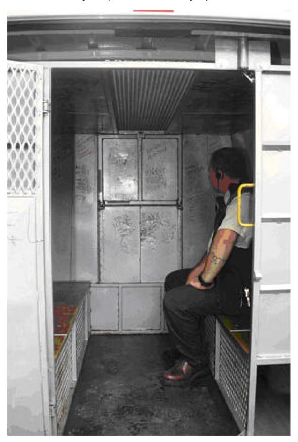
4. Interior rear cage with emergency exit hatch open
